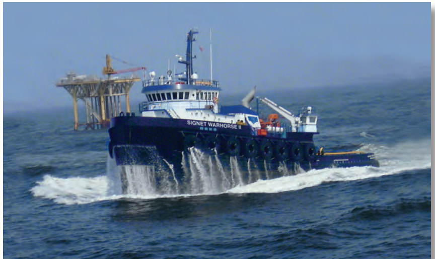
Demonstrating its strength, the SIGNET WARHORSE II, is the most powerful ABS classed ocean towing vessel in Signet Maritime's Offshore Towing Division. At 153.58 tonnes bollard pull, the SIGNET WARHORSE II will lead the fleet providing ocean towing of rigs, spars and other vessels.
